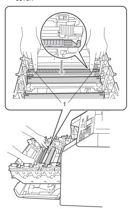
5 Clean the corona wire inside the drum unit by gently sliding the green tab from left to right and right to left several times.
